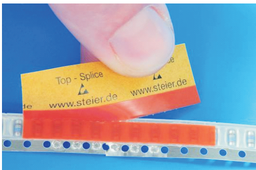
5.) tear along the micro perforation to remove the „handle“
